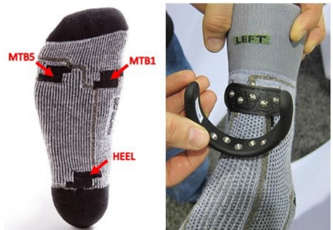
Figure 2. On the left the 3 proprietary textile pressure sensors located in key positions under the foot. On the right the socks' magnetic contacts for the attachment of the anklet.
